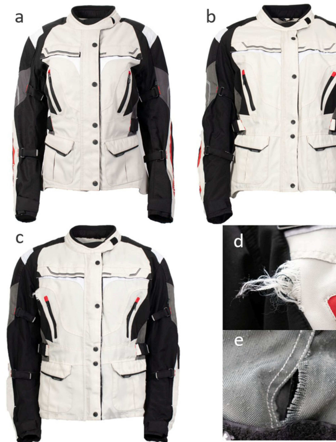
Figure 7. Textile jacket comparison. (a) new; (b) after 20 cold washing/line drying cycles; (c) after 10 hot washing/tumble drying cycles; and (d,e) points of seam failure after 10 hot washing/tumble drying cycles.
