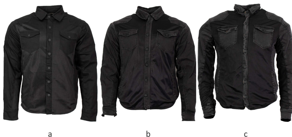
Figure 6. Photos of riding shirt: (a) new/no wash, (b) after 20 cold washing/line drying cycles and (c) after 10 hot washing/tumble drying cycles.
