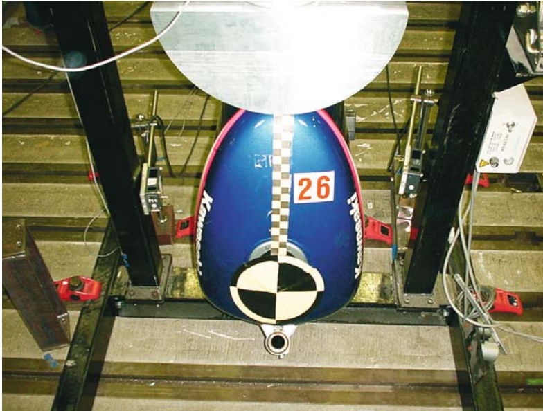
Figure 1. Set-up for performing a drop test for motorcycle fuel tank.
