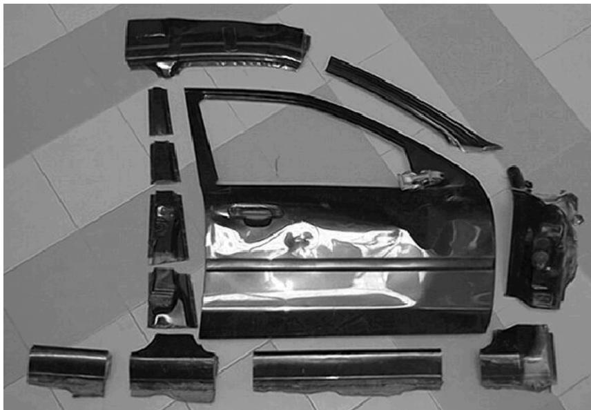
**Figure 5.10. Identification of beams' sections from a Mondeo car frame**
