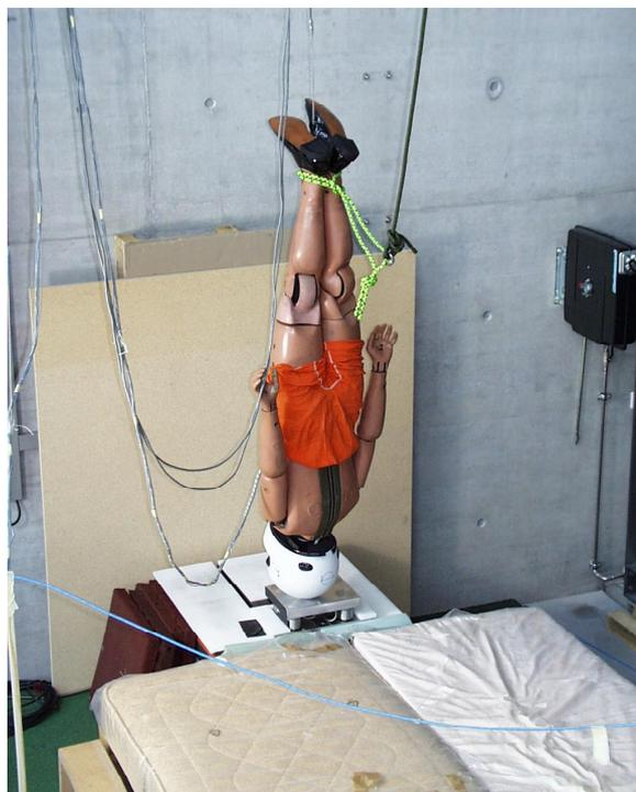
**Figure 8.9.** Experimental set-up for dummy drop tests: configuration for R/0°-impacts (left) and for P/90°-impacts (right).
