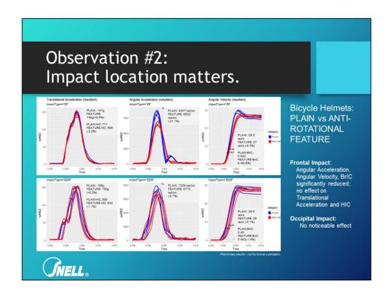
The first of these series compared results for bicycle helmets equipped with one of the popular anti-rotational innovations with similar, almost identical helmets without this feature. We noted a 20% reduction in peak angular acceleration for frontal impact although the results for angular velocity were remarkably similar. However, the results for the third site halfway between a rear and a lateral impact showed almost no difference at all.
