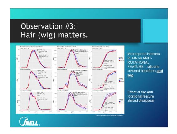
This next series was also conducted on helmets with and without the ant-rotational feature. The test head forms were all treated with silicone but also with a wig firmly in place atop the head form over the silicone coating. When the results were compared, there appeared to be no real difference. The wig broke the coupling between the head form and the helmet so completely that the anti-rotational feature had no effect on rotational acceleration or angular velocity in this series.
