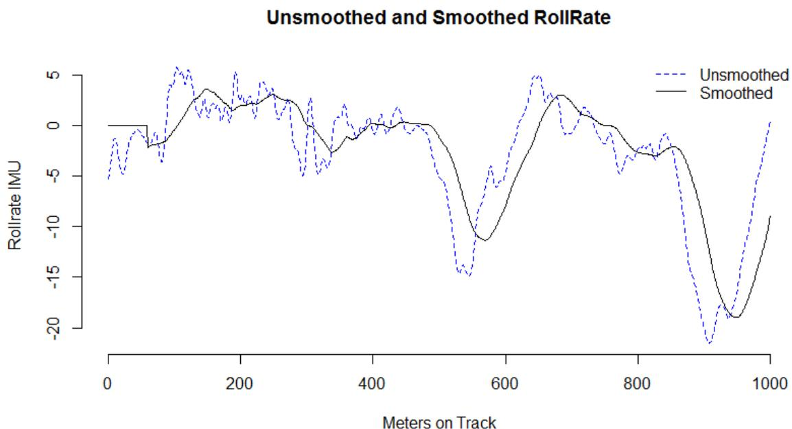
Figure 2: Example of the effect of smoothing and shifting the data (Rollrate in this case) of a single driver. We show only the first 1000 meters of the given ride. The “lag” between the rollmean and the actual data is well visible and this serves to ensure that critical dynamics affect the likelihood of the next few meters after their occurrence still (e.g. the potential recorded accident locations).
