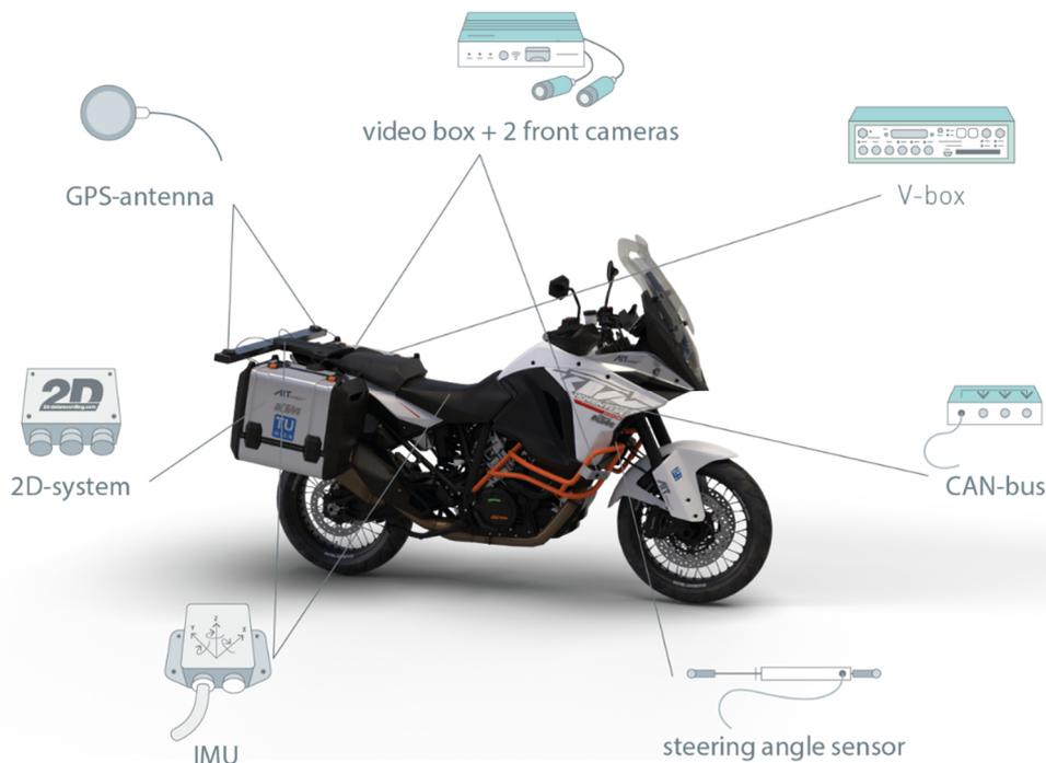
Figure 1: KTM 1290 Super Adventure equipped and instrumented as a Motorcycle Probe Vehicle (MoProVe)
