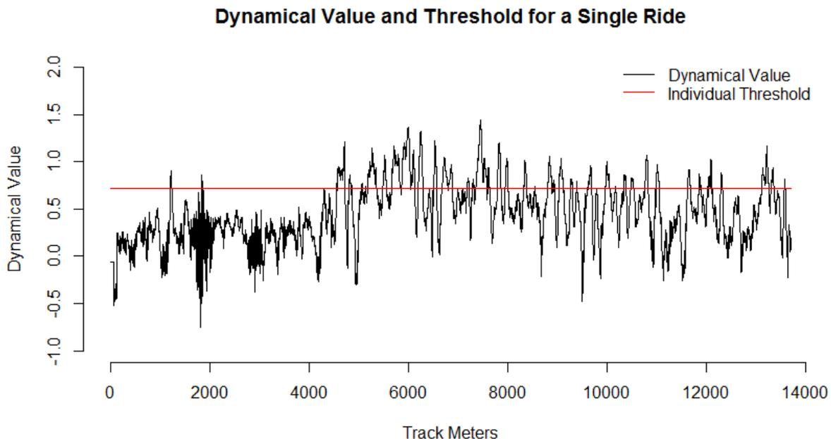
Figure 3: The measured dynamics on each meter of the track can be transformed into a value (“Dynamical Value”) that encodes whether dynamics might be in a similar risk domain as known accident spots. An individual threshold, derived from the Dynamic Values at known accident spots, allows to identify domains of interest for safety studies.
