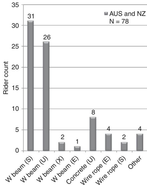
FIGURE 2 Barrier types and crash postures (1, 31) (S = sliding posture; U = upright posture; X = unknown posture; E = ejected).
