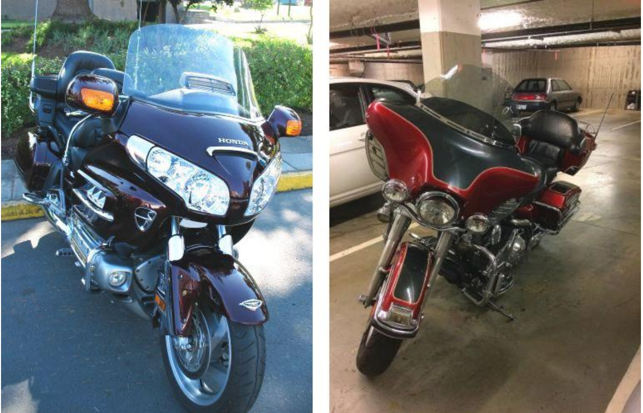
Figure 4: The large fairings on this Honda Gold Wing (left) and Harley Davidson Electra Glide (right) would render a fluorescent jacket ineffective. When viewed from the front, it is nigh-impossible to tell what a rider is wearing because their body is hidden behind the motorcycle's bodywork. Not all motorcycle fairings are this large, but because they are designed to protect the rider's body from the wind, they also obstruct the view an oncoming driver has of the motorcyclist's body; the only part of the rider that is always visible is the helmet.
