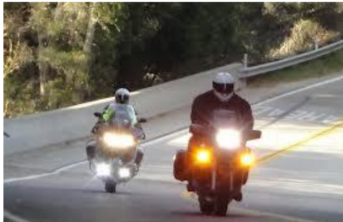
An example of auxiliary driving lights (white) and position/marker lights (amber). The available research indicates the larger triangular formed by the white driving lights is more noticeable.
