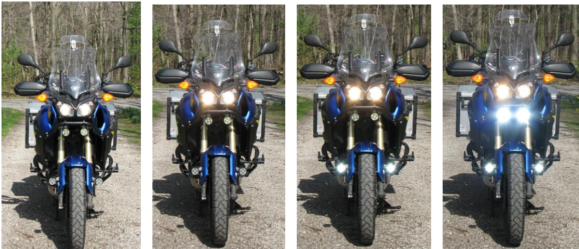
Pictures: left to right – (1) stock headlight on dim, (2) bright, (3) bright with lower set of auxiliary lights, (4) bright with lower and upper set of auxiliary lights
