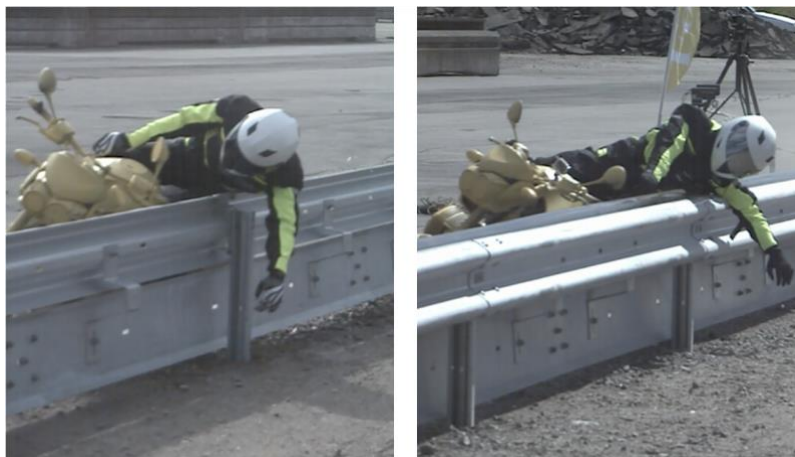
Figure 18: Upright crash tests into a W-beam barrier at 60 km/h at 10° impact angle, without top protection (left) and with top protection (right). Source Folksam (2015a).
