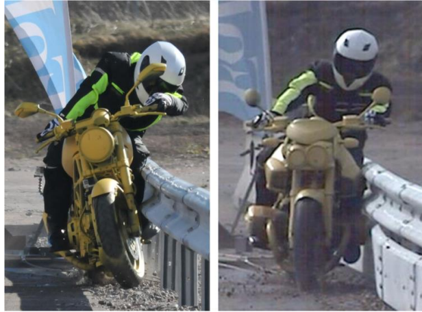
Figure 16: Crash tests into a W-beam barrier at 60 km/h at 10° impact angle with a conventional motorcycle (left) and a boxer-engine motorcycle (right). Source: Folksam (2015a)
