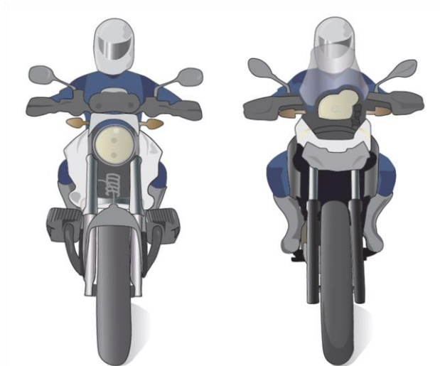
Figure 10: A front-view illustration of a motorcycle equipped with a boxer-twin engine (left) and a similar one with a single-cylinder engine (right).
