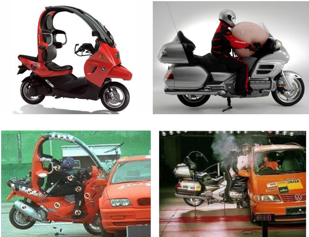
Figure 9: The BMW C1 (left side) and the airbag-fitted Honda Goldwing 1800 (right side). Source of crash test pictures: BASt (BMW C1) and ADAC (Honda Goldwing).
