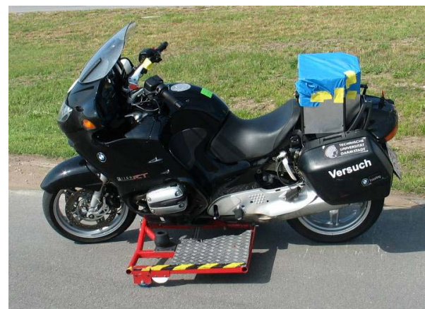
Figure 1. Test motorcycle BMW R1150RT; during braking tests with integrated and hidden measurement instrumentation and outriggers to limit damage in case of a fall
