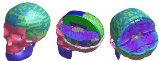
Figure 7 The ESI H-Head finite-element model.
