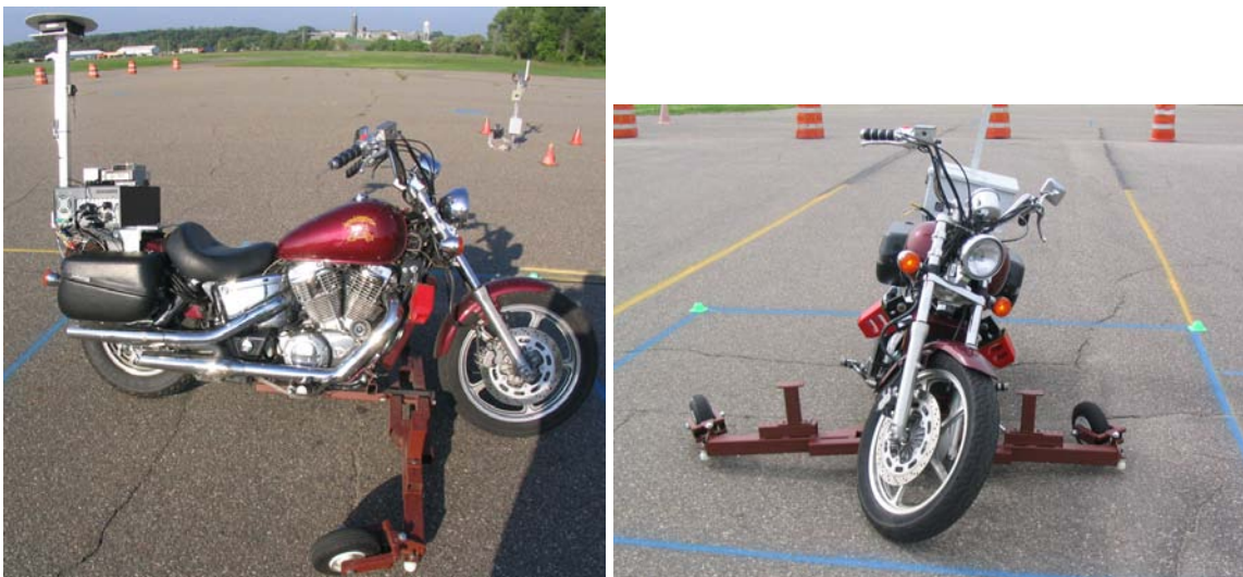
Figure 3. Pictures of the instrumented test motorcycle, a 2000 Honda Shadow VT1100.
