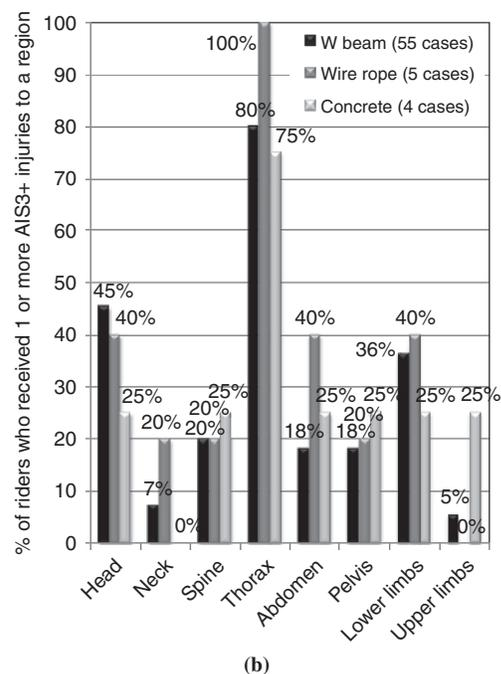
FIGURE 3 Injury profiles for (a) crash postures in collisions with W-beams and (b) barrier types in all crash postures (1).
