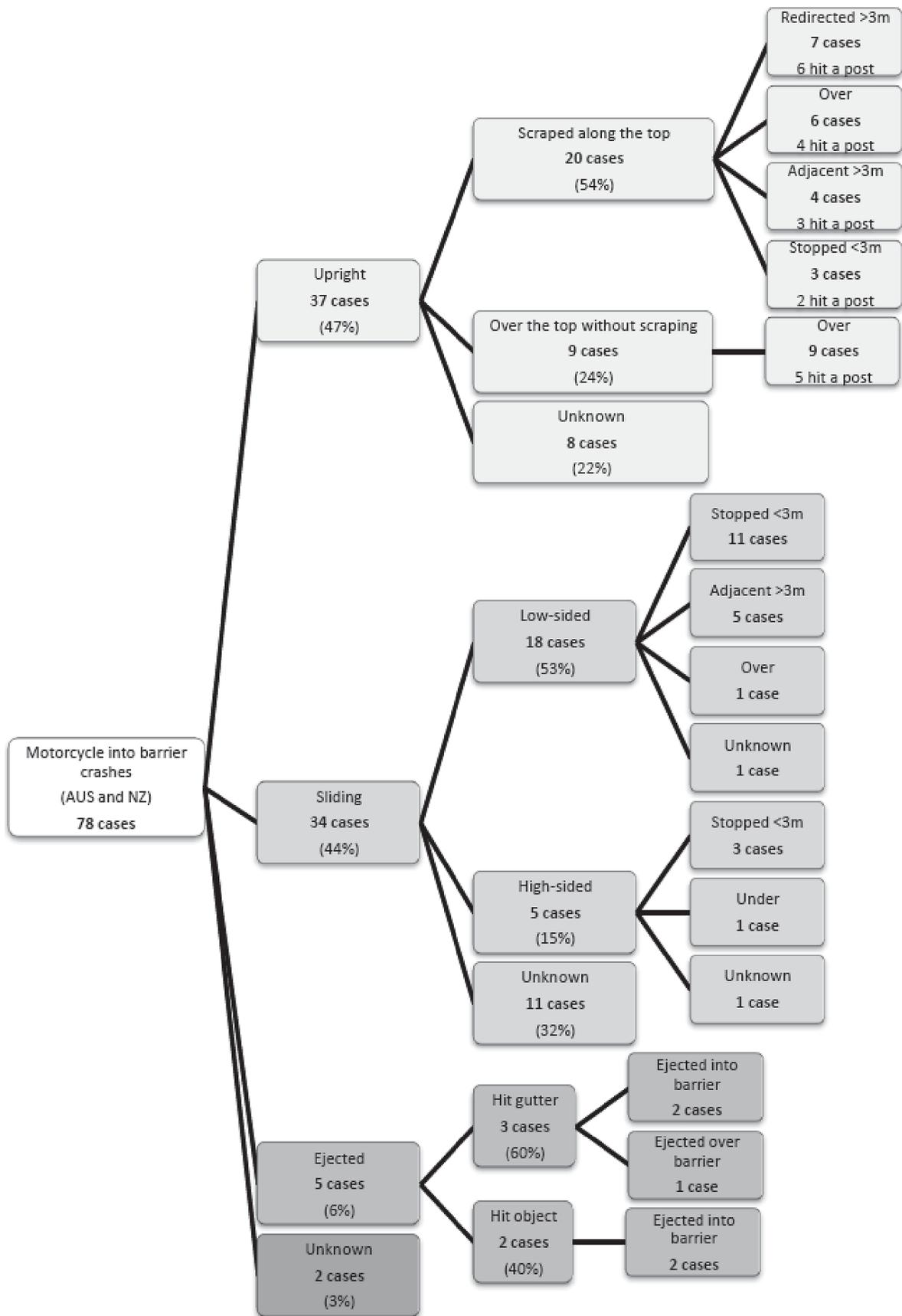
FIGURE 1 Crash modes, motorcyclist kinematics, and guardrail impacts with post for 78 motorcycle-into-barrier impacts (AUS = Australia; NZ = New Zealand) (1, 31).
