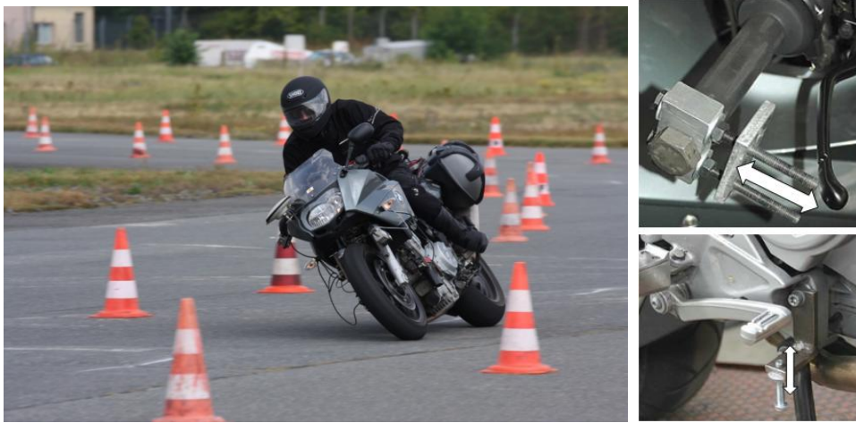
Figure 9: BMW F800S test bike equipped with measurement devices and manually adjustable brake lever stops during corner braking experiments.
