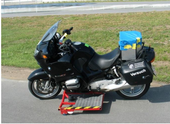
Figure 3: Test motorcycle equipped with outriggers
