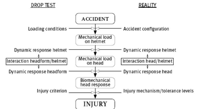
Figure 3 Load-injury scheme for helmeted head impact (van den Bosch [20] modified from Wismans [21])
