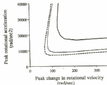
Figure 2. Diffuse axonal injury rotational acceleration and rotational velocity thresholds for infant (500g brain mass, heavy solid line) and adult (1067g brain mass, solid line, 1400g brain mass, dashed line) [18].
