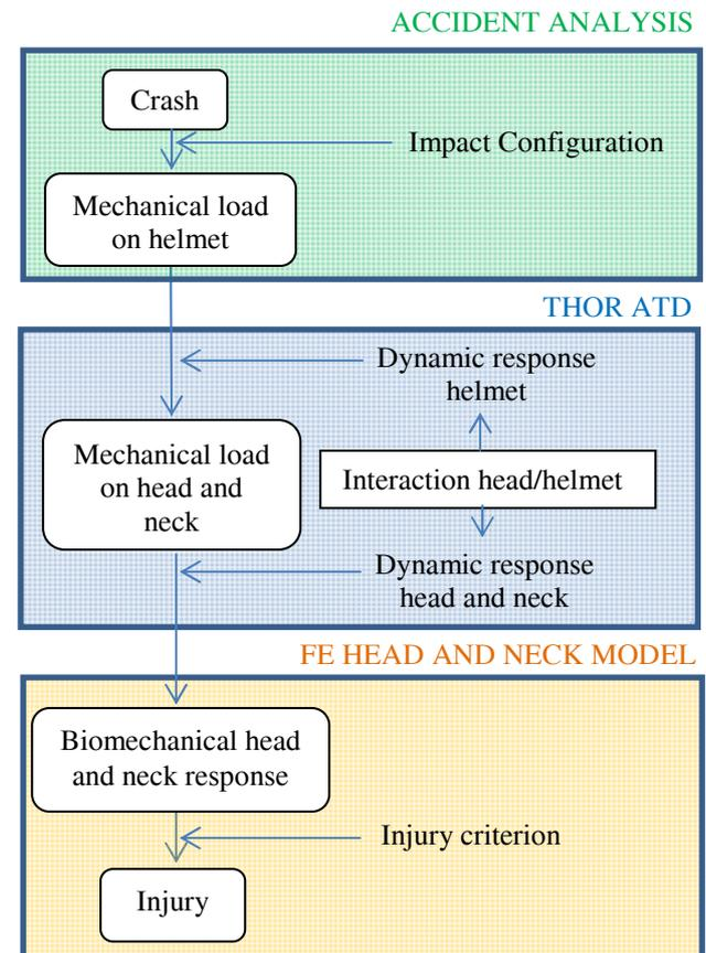
Figure 5 The investigation methodology for the project demonstrating the use of the THOR dummy head and neck and the finite element model.
