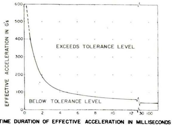
Figure 1. The Wayne State University Concussion Tolerance Curve for linear acceleration, after SAE (1980) [16].
