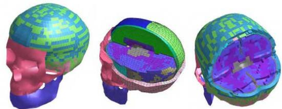
Figure 7 The ESI H-Head finite-element model.
