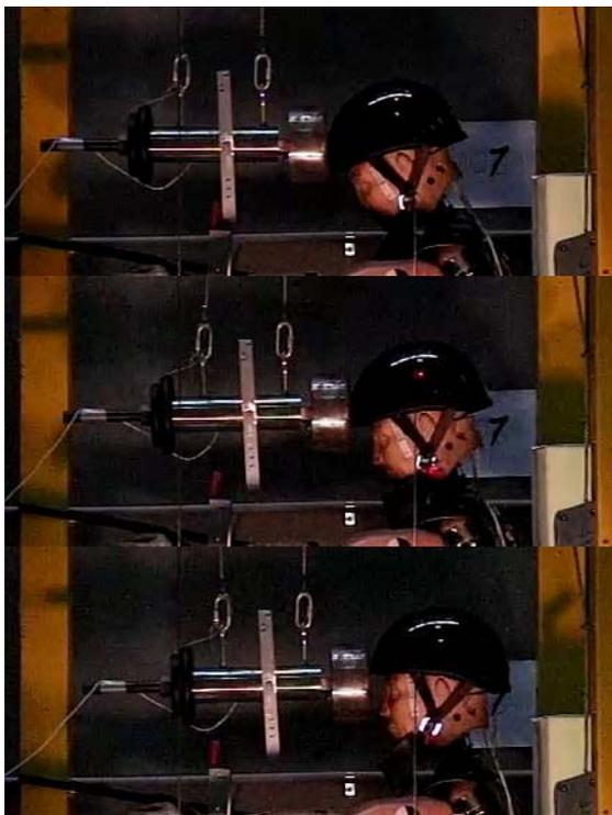
Figure 6 A helmeted THOR head and neck responding to a pendulum impact to the head.
