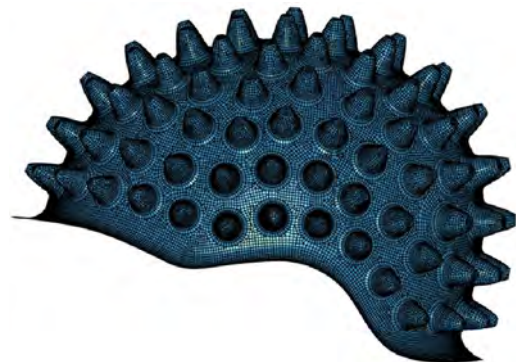
Fig. 11. ABS cone liner proposed by Blanco et al. (2010).
