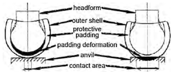
Fig. 9. Helmet deformation modes with FRP (left) and PC (right) shells (Beusenberg and Happee, 1993).
